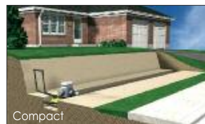
Install drain pipe, wall rock and level
